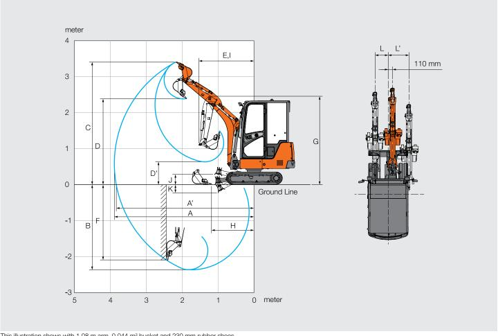
This illustration shows with 1.08 m arm, 0.044 m³ bucket and 230 mm rubber shoes.
